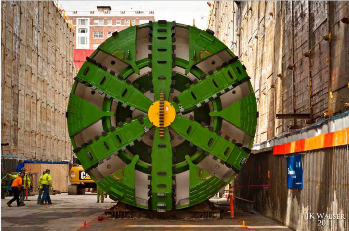
Figure 21. Example of a Tunnel Boring Machine
