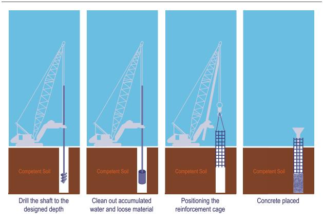
Figure E-1 Drilled Shaft Foundatioin Construction
