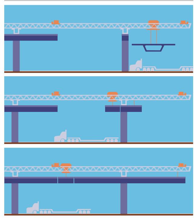
Figure E-4 Balanced Cantilever Construction Stations
