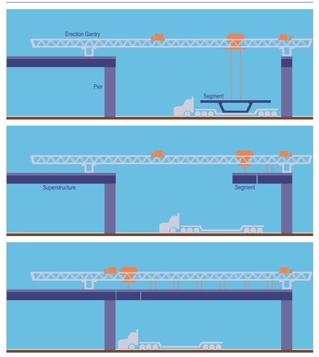
Figure E-3 Segmental Precast Bridge Construction
