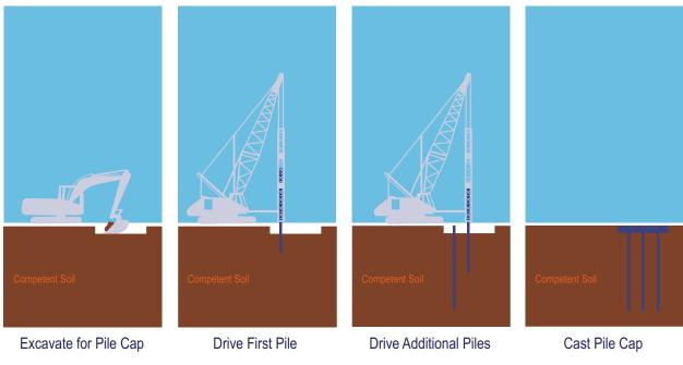
Figure E-2 Driven-pile Foundation Construction Piers
